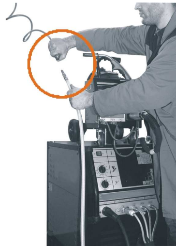
5 - Connect compressed air tube of carbon electrode holder to air supply. Min. pressure 5 bar, min. flow 100 lts/min.
