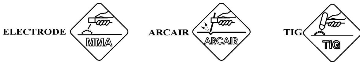
300, 400, 500, 600 models allow TIG welding process due its extraordinary adjustment range. With a TIG economizer (equipped with gas valve and socket for TIG torch connections) installation or High Frequency generator, it is possible TIG welding even in mild and stainless steel plates from 0,6 mm thick.
